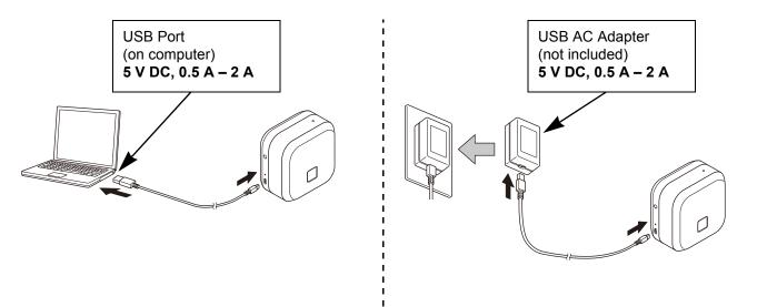
Connect the label printer to the computer using the included USB cable, or connect the USB cable to a USB AC Adapter suitable for charging mobile devices, and plug the adapter into a power source. Charge until the Battery LED turns off.
